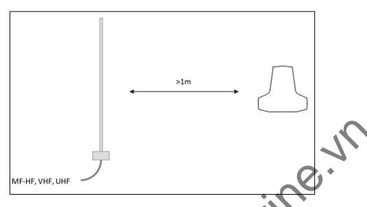
1.1.4 The antenna unit should be installed with a 360° clear view of the sky. However, minor obstructions such as a mast will not degrade the antenna performance severely, if a separation distance larger than 15 times the diameter of the obstruction is kept.
