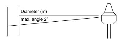
1.4.2.2 If two Inmarsat-C antennas are installed, the vertical distance between them should be at least 1 metre to eliminate interference. The antennas should be installed such as to ensure electromagnetic compatibility.
